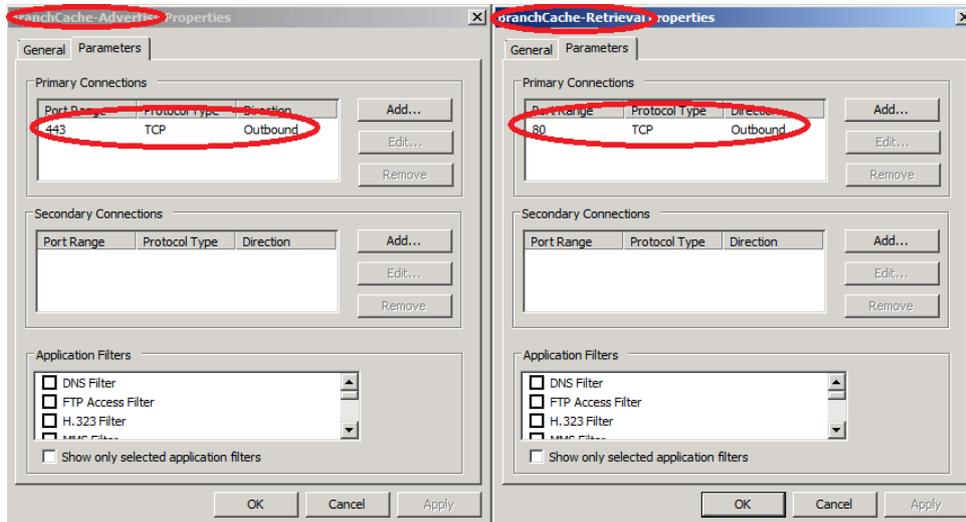
After the new Protocol definitions have been created we must create two new Firewall rules which allows traffic for these protocol definitions from the internal network to the Localhost Network and vice versa.
