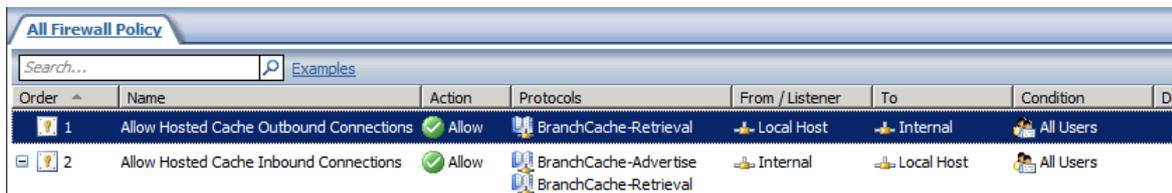
Figure 6: firewall rules for BranchCache
