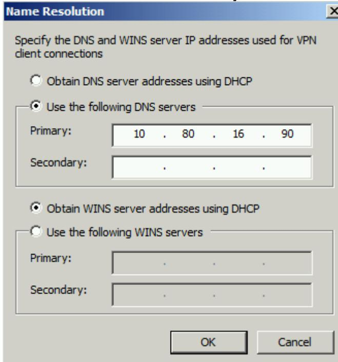
Figure 4: Name resolution for SSTP clients
