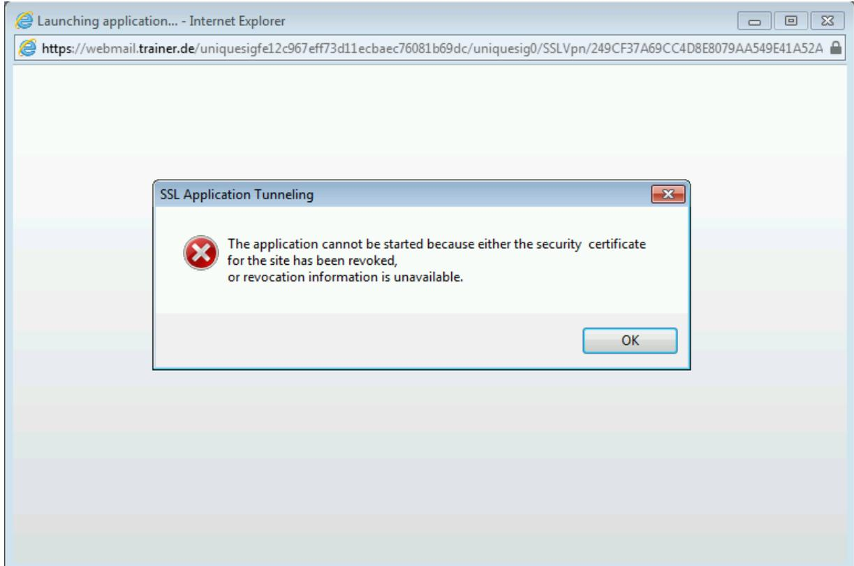
Figure 12: SSTP certificate revocation check failed
