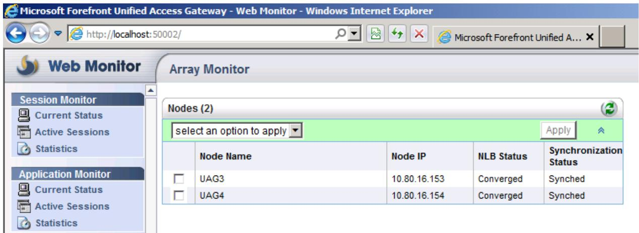
Figure 7: NLB is converged
