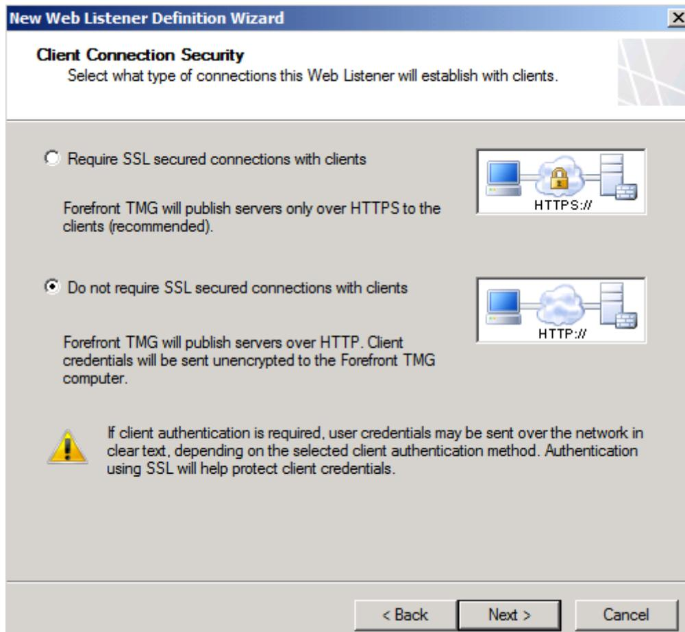
Figure 8: Connect via HTTP
