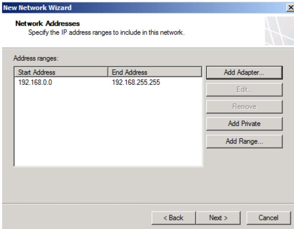
Figure 12: Forefront TMG – IP address ranges
