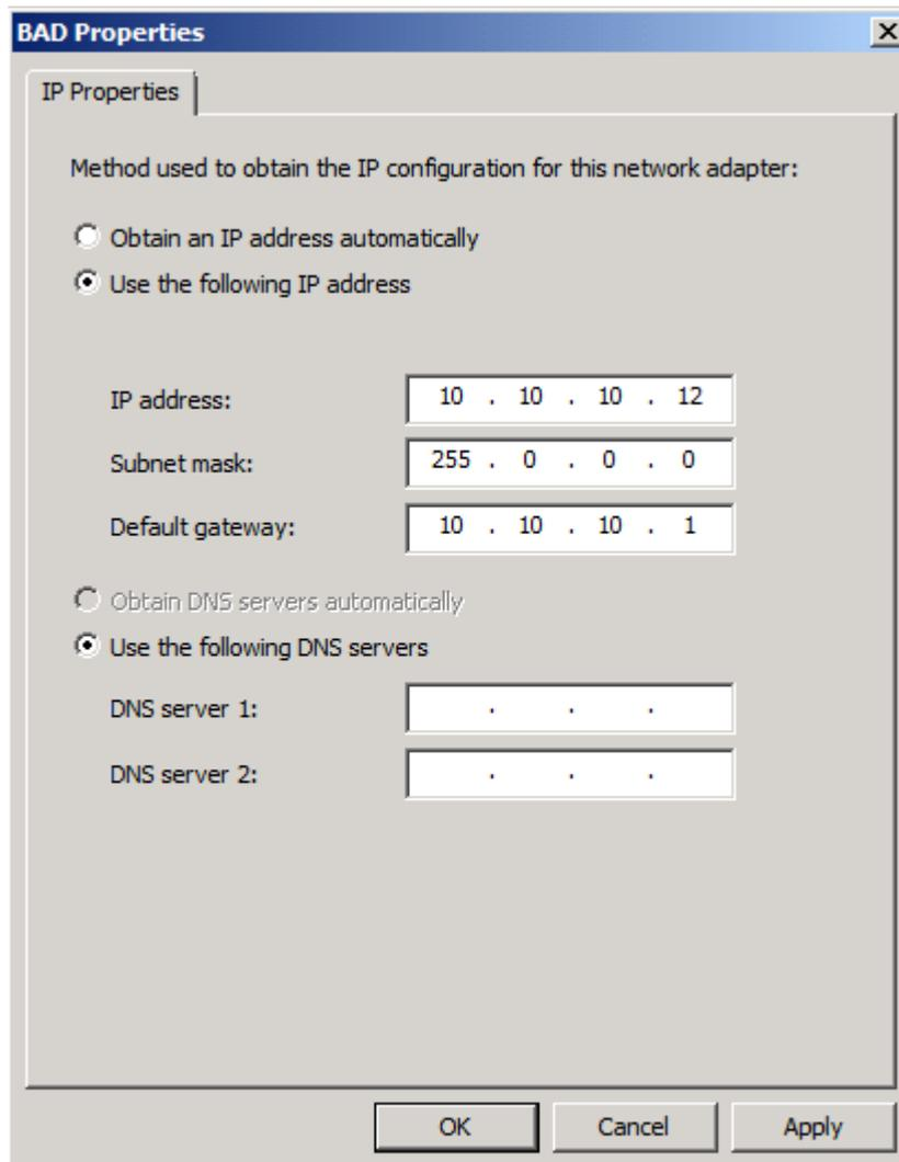
Figure 7: Forefront TMG IP address properties
